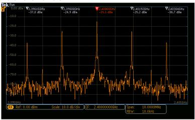
Automatic Markers identify spectral peaks, with the reference marker assigned to the highest amplitude peak. Manual Markers can also be used to investigate other areas of interest in the spectrum or to measure phase noise and noise density.
