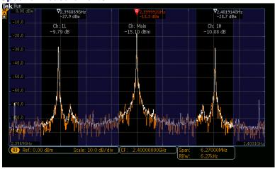
Typical spectrum analyzer measurements are supported, including Channel Power, Adjacent Channel Power Ratio, and Occupied Bandwidth
