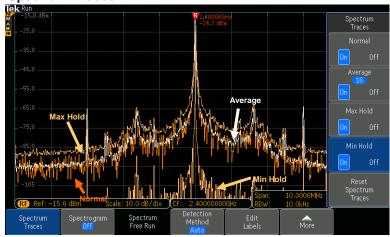
Unlike traditional FFT, the MDO3000 supports typical spectrum analyzer traces: Normal, Average, Max Hold and Min Hold.
